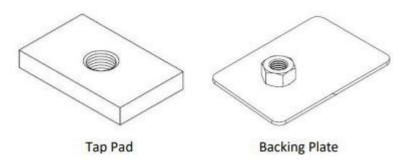
4.23 With all the roll cage mounting plates in position they can be tack welded to the shell at 3 or 4 locations on each plate.
